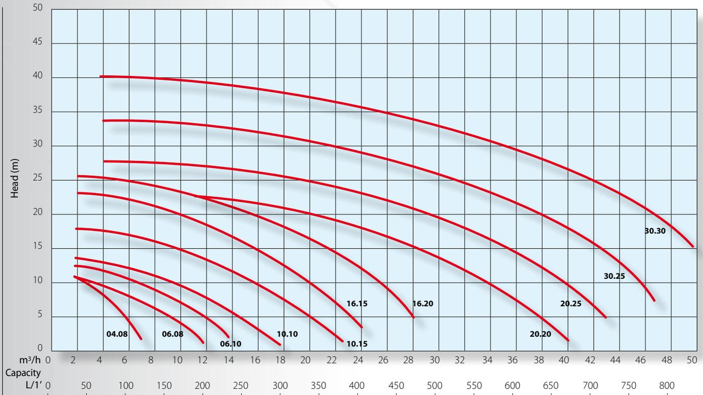
NOTES: All curves are referred to: water at 20°C - viscosity 1 °E - specific gravity 1 kg/dm³ pt
