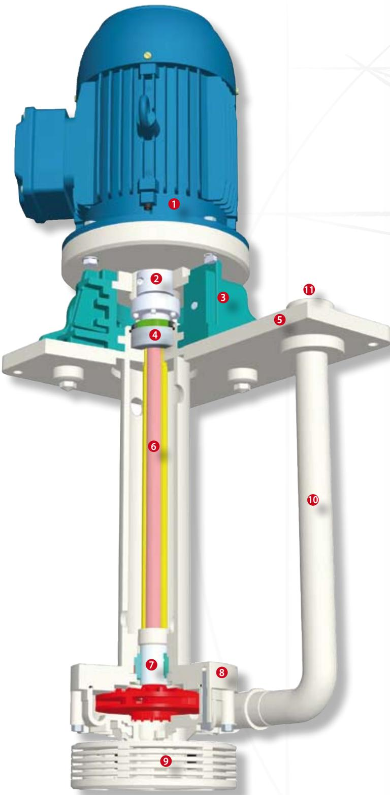
**KME** - Constructed for fixed installations with the pump body immersed in basins, tanks, collecting wells, reservoirs. Fluids with a specific gravity of 2 kg/dm<sup>3</sup> can be handled in function of installed power, with a kinematic viscosity max. of 75 cSt and temperatures as detailed in the table 2
