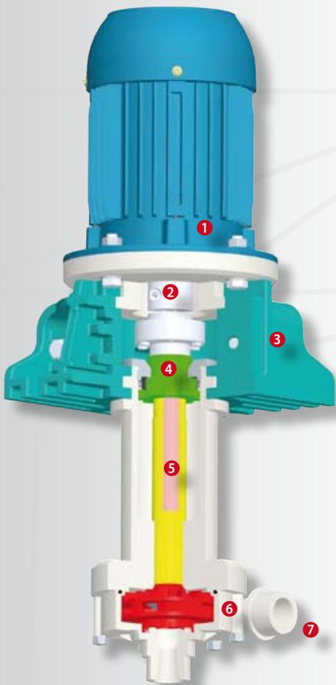
**HME** - Constructed for fixed installations, with the pump body submerged in basin, tanks, collecting wells, and for those with supports external to the container of the liquid. In this case, a secondary discharge pipe is required, between the pump and the container of liquid, set on the pump column. (Fig. A)
